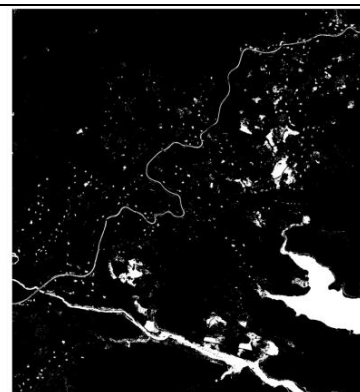
Figure 3.8: Extracted patches of tar road after removing vegetation areas
